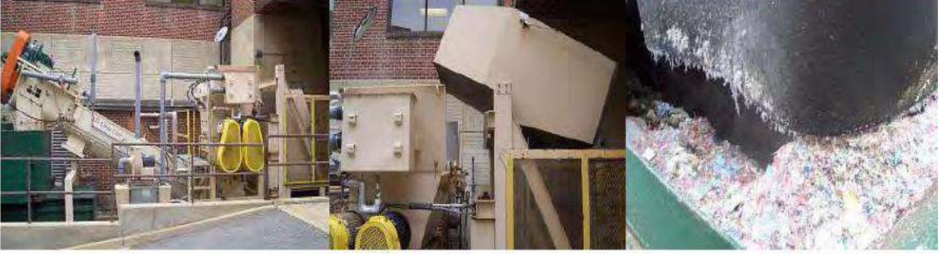
STI ChemClav (L), automatic waste dumper (M), and close-up of treated/shredded waste (R)
