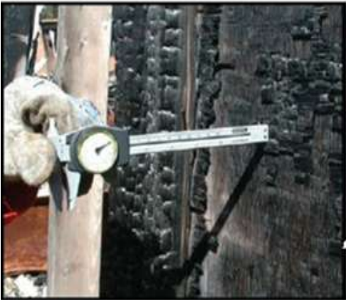
(b) Using Dial Calipers to Measure Depth of Char.
