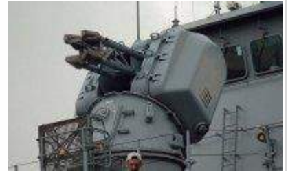
Oerlikon Contraves Sea Zenith 25mm CIWS system×3
