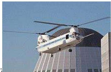
CH-47B used as an in-flight simulator at Moffett Field. It was formerly used by the U.S. Army, under number 66-19138.
