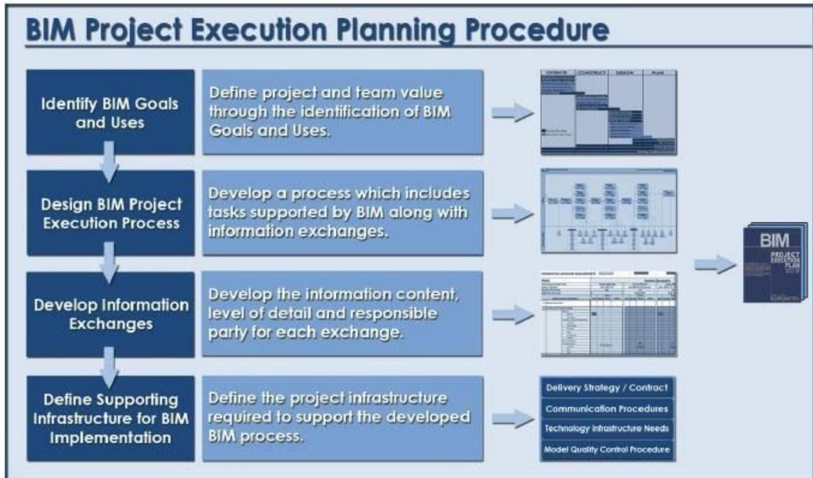
Figure i-1: The BIM Project Execution Planning Procedure
