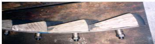
Example of bolted liners
