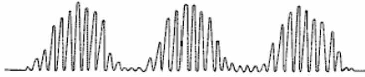
HALF-WAVE RECTIFICATION OF ABOVE SIGNAL
