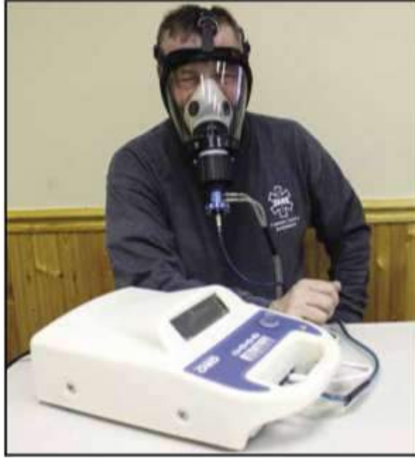
A firefighter undergoing SCBA facepiece fit-testing.
