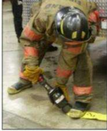
Attaching nozzle, stepping on hose
